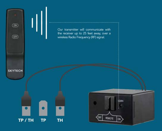
Underneath the fireplace, you will find a valve that will have these three terminals on it: TP/TH, TP, and TH. The receiver wires will connect to the TP/TH and the TH terminals.
